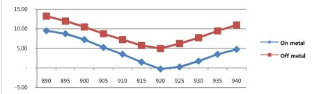
•TRAY U reads shorter by 30% or less off metal (or on non metal surface). With still reading 2.0 meters off metal, It can be applied for BOTH metal and off metal application.
