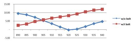
•TRAY U reads best without any metal bolt in two holes (located diagonal directions). With RF interference, metal bolts decreases read range by 50% or more. RFcamp recommends not using metal bolts, but 3M 300LSE adhesive or glue for maintaining optimum read performance. In case adhesive or glue can not be used, polycarbonate (or nylon) bolts is recommended.
